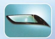
On the glass surface to be printed conductors using silver paste with a special pattern. This will serve as conductor antenna to receive radio signals to the audio player in the Car so you no longer need regular antenna and will add value aesthetic beauty of the car. These antennas can be implemented on glass rear and side window glass.
